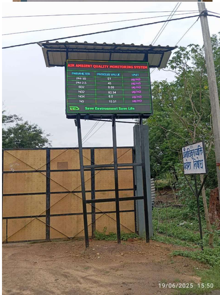
Figure – 4 Online monitoring systems for ambient air quality
